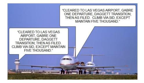
**Note:** Standard Instrument Departure (SID): A preplanned instrument flight rule (IFR) air traffic control (ATC) departure procedure printed for pilot/controller use in graphic form to provide obstacle clearance and a transition from the terminal area to the appropriate en route structure.
