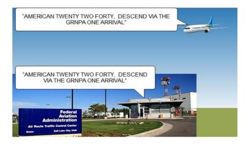
**Note:** Standard Terminal Arrival (STAR): A preplanned instrument flight rule (IFR) air traffic control arrival procedure published for pilot use in graphic and/or textual form. STARs provide transition from the en route structure to an outer fix or an instrument approach fix/arrival waypoint in the terminal area.
